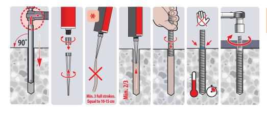
\* Squeeze out separately a minimum of 3 full strokes (Equal to 10-15 cm ) until the mortar shows a consistent colour.
