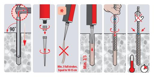
\* Squeeze out separately a minimum of 3 full strokes (Equal to 10-15 cm ) until the mortar shows a consistent colour.
